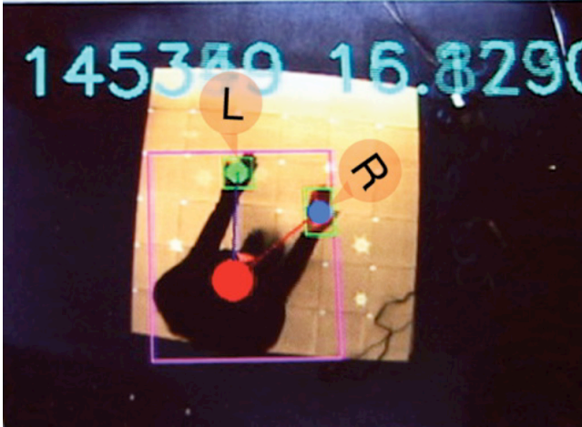
Figure 7. Image recognition results. Red circle: center-of-mass of a user's body, green circle: left palm orientation, blue circle: right palm orientation.
