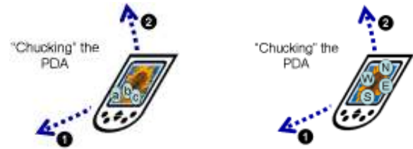
Figure 4. Chucking and Flicking benefit touch input modes, for (a) specifying the position of the object on the public display, and for (b) identifying the orientation of the object.
